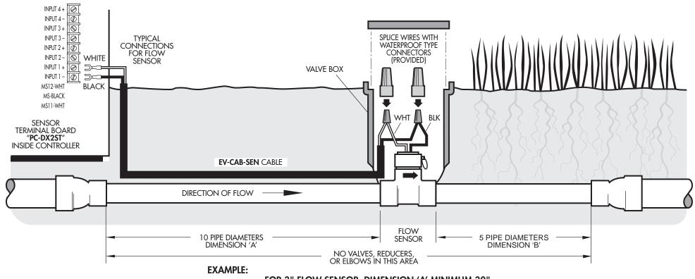
FOR 3" FLOW SENSOR, DIMENSION 'A' MINIMUM 30" **DIMENSION 'B' MINIMUM 15"**
