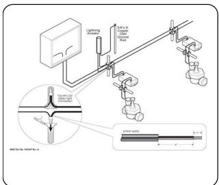
STEP 4: Connect 2-wire cable to controller
