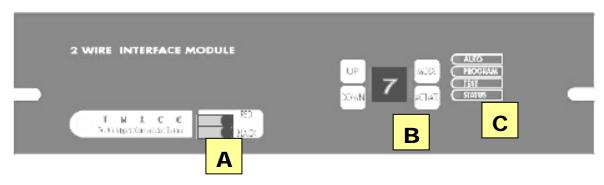
The Connector [A] is used for assigning Station # to Decoders
