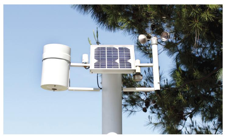
A swater resources become more critical, the demand for "weather-based" control of irrigation systems has increased significantly. Therefore, an "onsite" weather center is the preferred means of weather monitoring, as it provides the ability to access the specifics of the local "microclimate" being irrigated.
