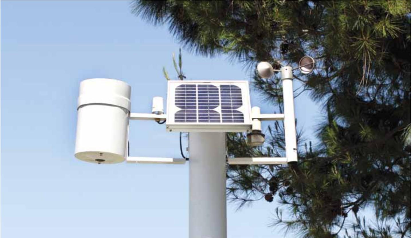
**A**s water resources become more critical, the demand for “weather-based” control of irrigation systems has increased significantly. Therefore, an “onsite” weather center is the preferred means of weather monitoring, as it provides the ability to access the specifics of the local “microclimate” being irrigated.
